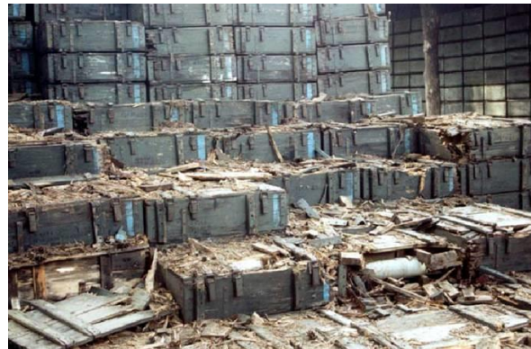
Figure: A deteriorating open-air AXO dump. Since these munitions were temperature-cycled over long time, typically they cannot be cleared by moving, but should be detonated in situ . (Photo courtesy OSSE)
