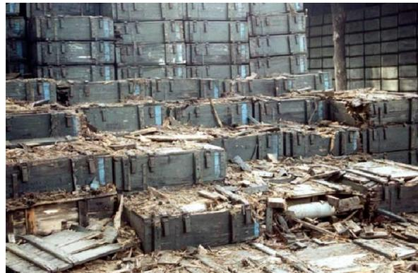
Figure: A deteriorating open-air AXO dump. Since these munitions were temperature-cycled over long time, typically they cannot be cleared by moving, but should be detonated *in situ*. (Photo courtesy OSSE)
