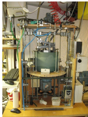
Wear tester for testing hardened steel used in expansion of liner pipes
